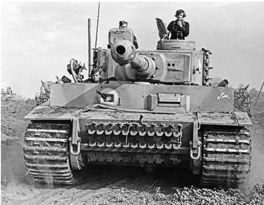
The legendary Tiger I heavy tank was a formidable weapon on the Eastern Front. The impenetrable armor, powerful 88mm gun, and huge size of the Tiger made it a legend in its time. The frontal armor was 100 mm thick, making it virtually impervious to Soviet guns.
